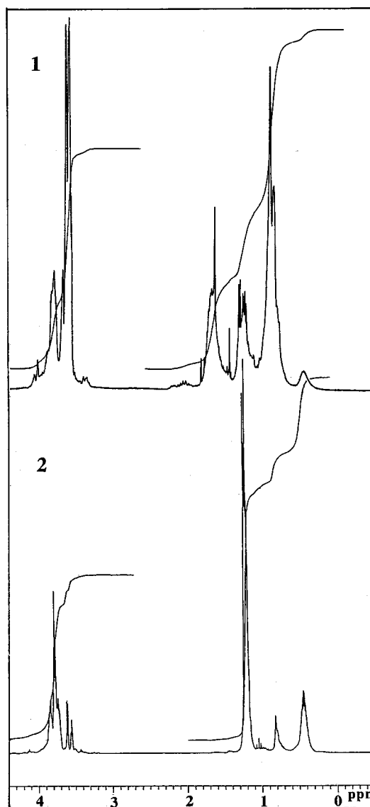
Figure 2. ^1\text{H} NMR spectra of polymers 1 and 2 obtained using the radical initiator (AIBN) and the anionic catalyst ( \text{LiAlH}_4 ), respectively.
